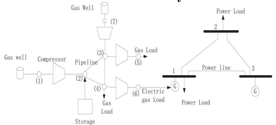
**Fig. 3 Coupled 7-node Natural Gas and 3-node Power Systems.**
