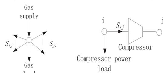
**Fig. 2 Gas Flow and Compressor Model.**
